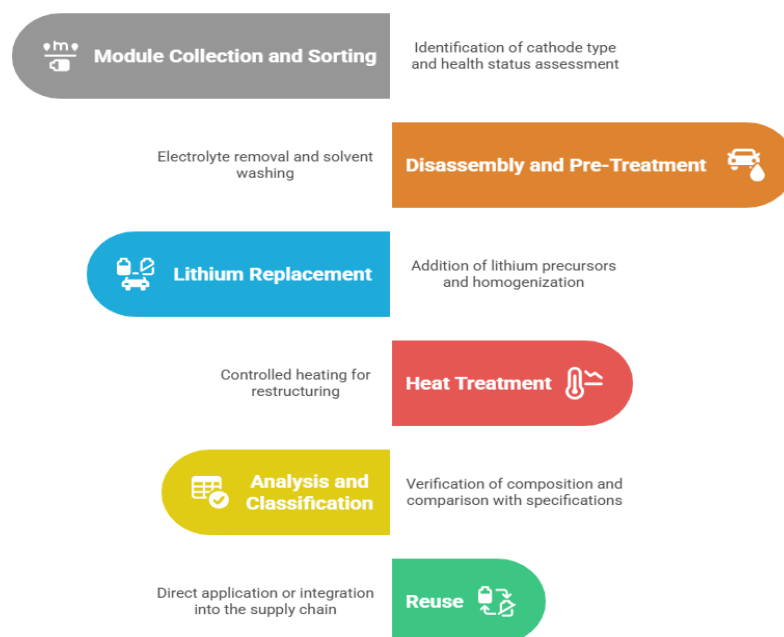
Figure 1. Key steps of direct cathode regeneration in lithium-ion batteries.
